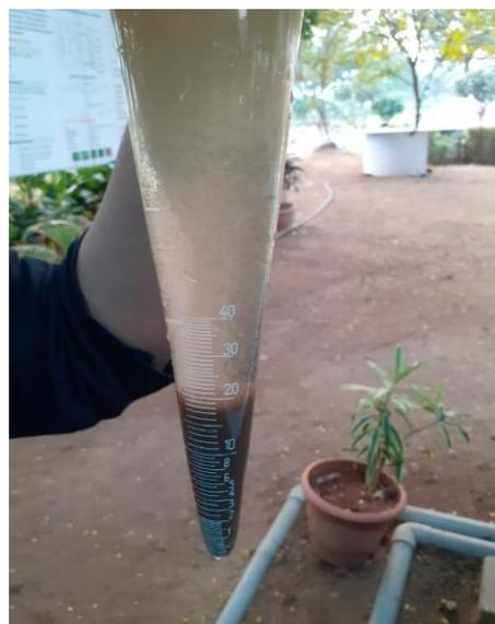
Floc volume measurement with Imhoff cone
